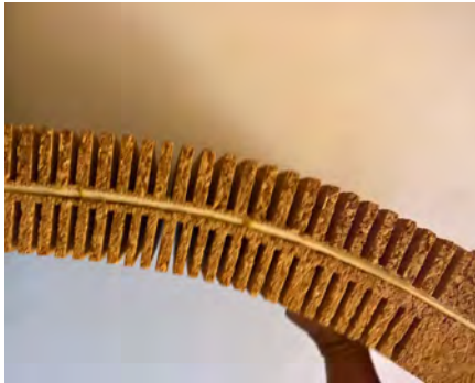
Bending Ply Too stiff, begins to crack. Cannot achieve correct degree of bend.
