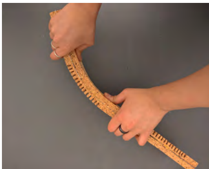
Shade Cloth Tough to bend – Less stiff than Bending ply. However, cannot achieve desired bend.
